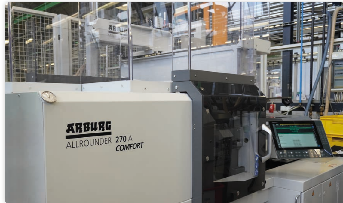
The fully electric Arburg 270 A with a freely programmable 3-axis robot
